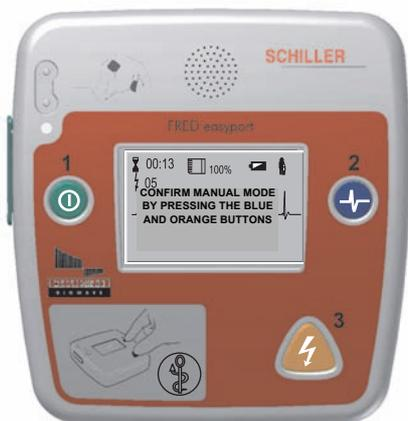
1. Switch the device on by pressing the green button (1).
